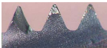
従来品 10穴加工後 Conventional after threading 10 holes.
